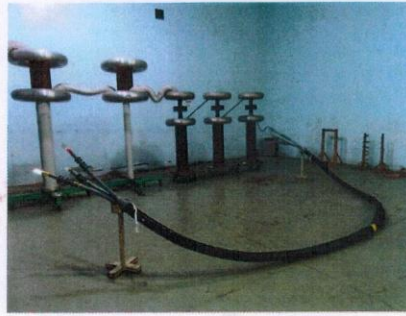
F2: 样品局部放电试验及交流耐压试验 Partial discharge test and AC voltage test on the sample
